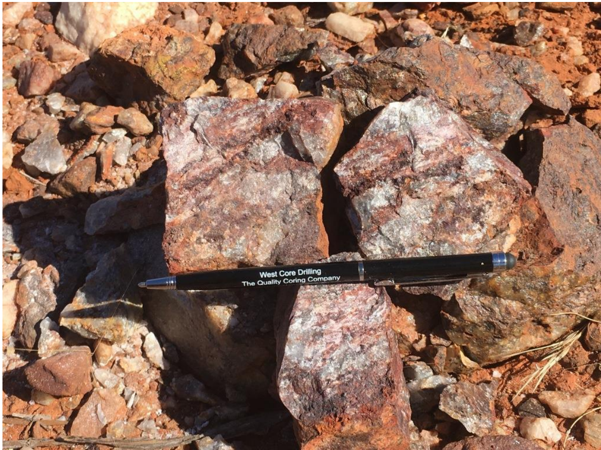
Figure 4: Fenceline Gold Prospect - close up photo of ferruginous vein quartz material (Sample WW170605) - where assays returned 3.01g/t gold.
