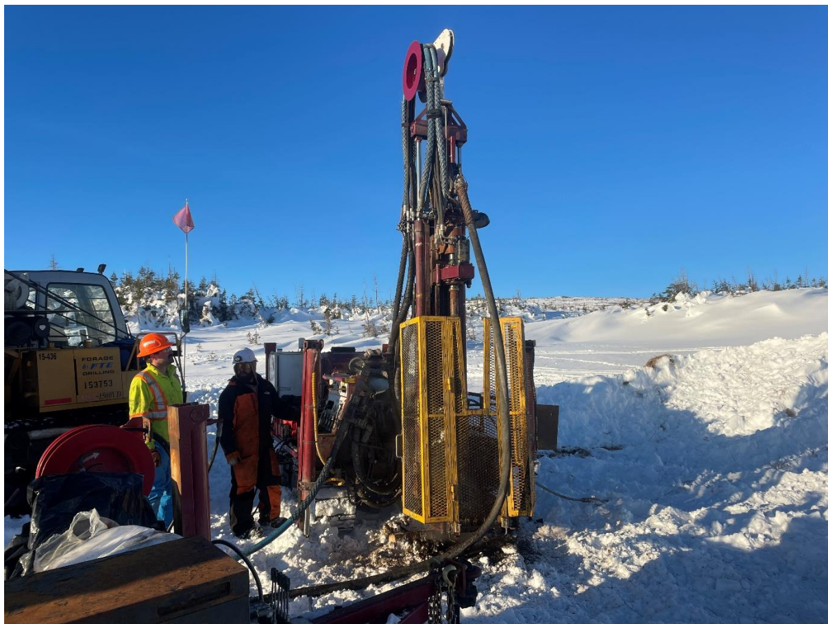
FIGURE 2: RC DRILLING AT O-2 TARGET AT MALACHITE 3
