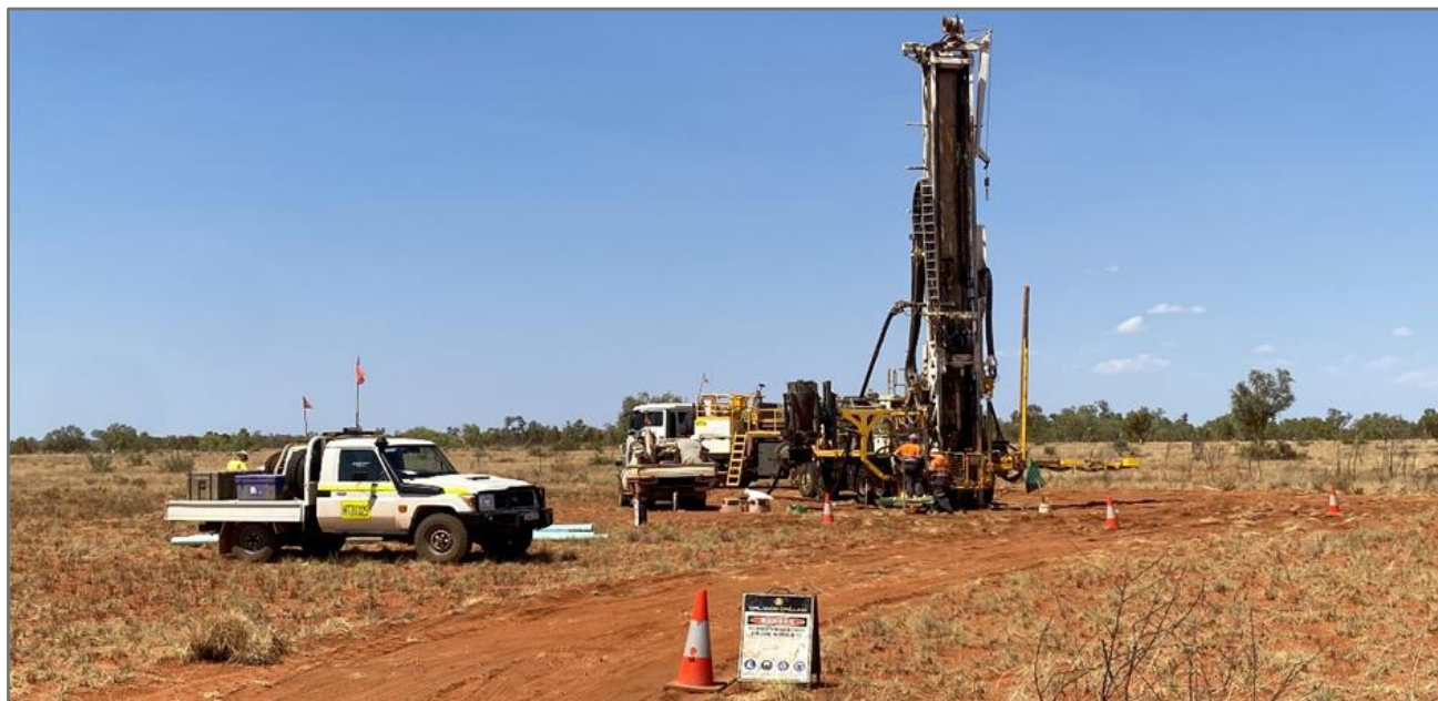
Figure 8: Photo of RC Drill Rig onsite at Quartz Hill.
