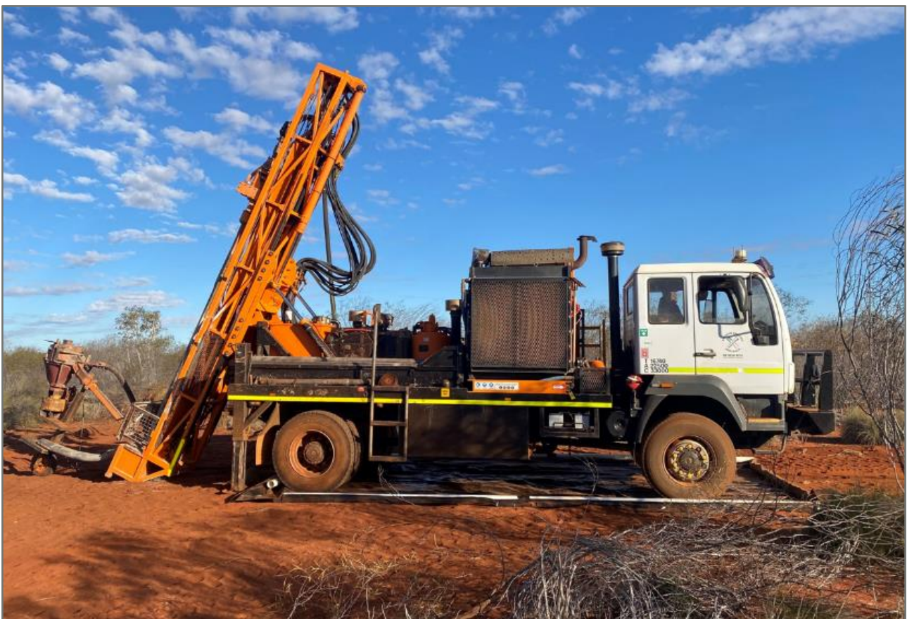
Figure 5: Air Core rig primed to drill NAE's first exploration hole at Wagyu Gold Project.
