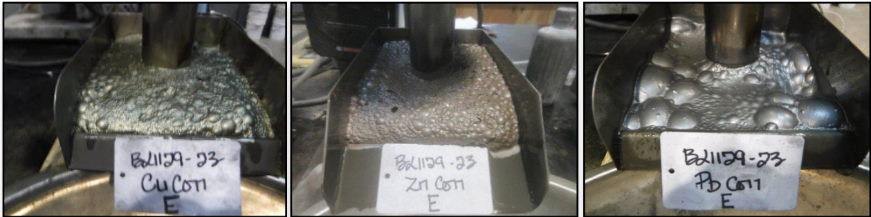
Figure 9. Photos of Copper, Zinc and Lead-Silver concentrate from Locked Cycle Testing
