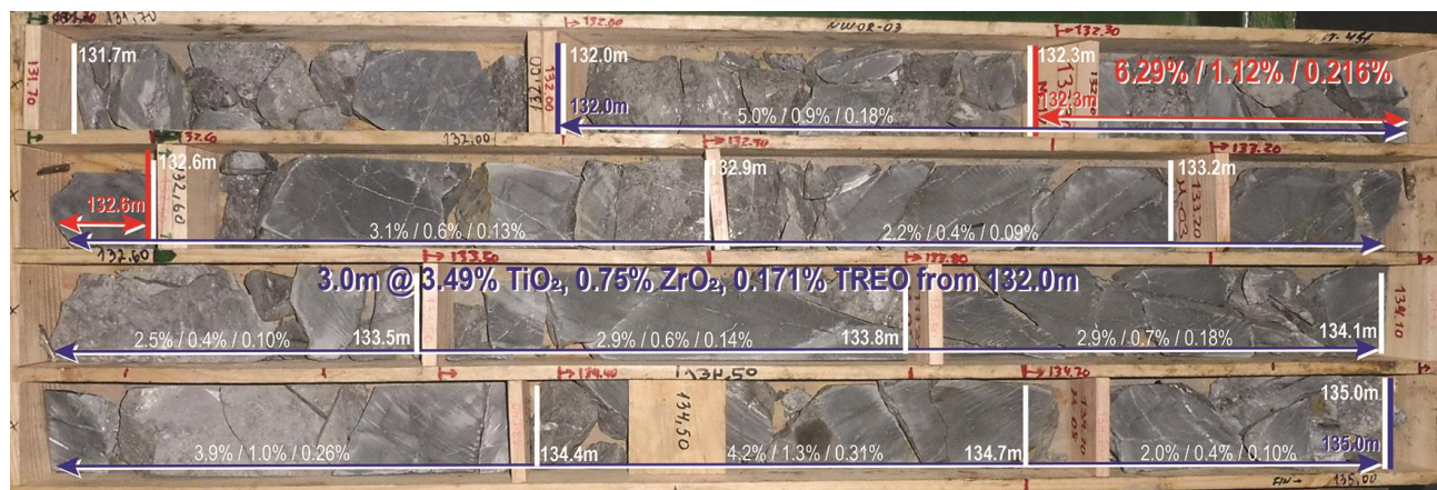
Figure 3 – NWOR-03 core photos with individual grades (white; TiO 2 % / ZrO 2 % / TREO%) and weighted average assay grades (blue: 2.0% TiO 2 cut-off; red: 5.0% TiO 2 cut-off).
