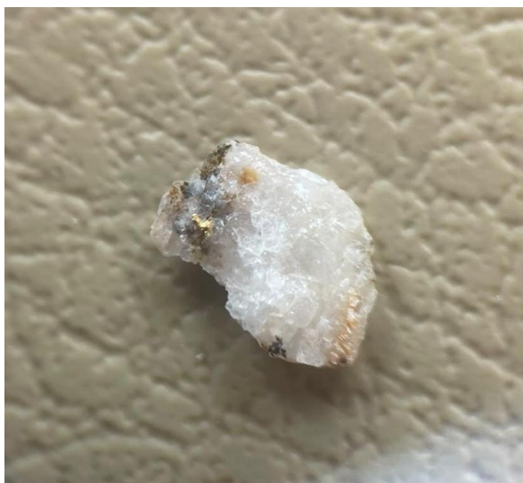
Figure 4: Visible gold under 10x magnification. Sample assayed 10.6 g/t gold
