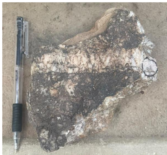
Figure 5: Location of visible gold highlighted in black circle within narrow vein cross-cutting an earlier brecciated quartz vein. (Sample L156090)
