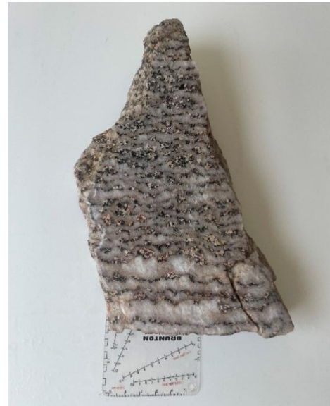
Figure 8: Interpreted highly fractionated magmatic indicators, UST banding from outcrop.
