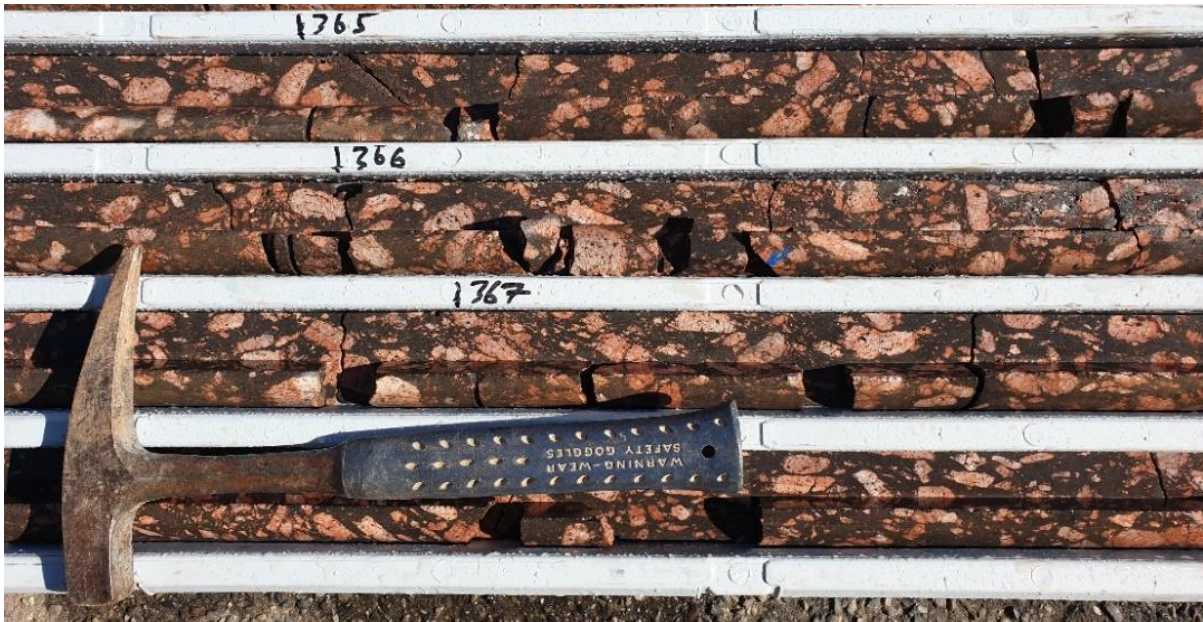
Figure 1 – Hole ID MCDA5-01 – Photo of core tray box 52, showing a portion of the breccia sequence. The dark matrix comprises iron-oxide enriched sericite-biotite. Clasts comprise coarse K-feldspar from the local host granite. Breccia matrix is enriched in the light rare earths, cerium and lanthanum.
