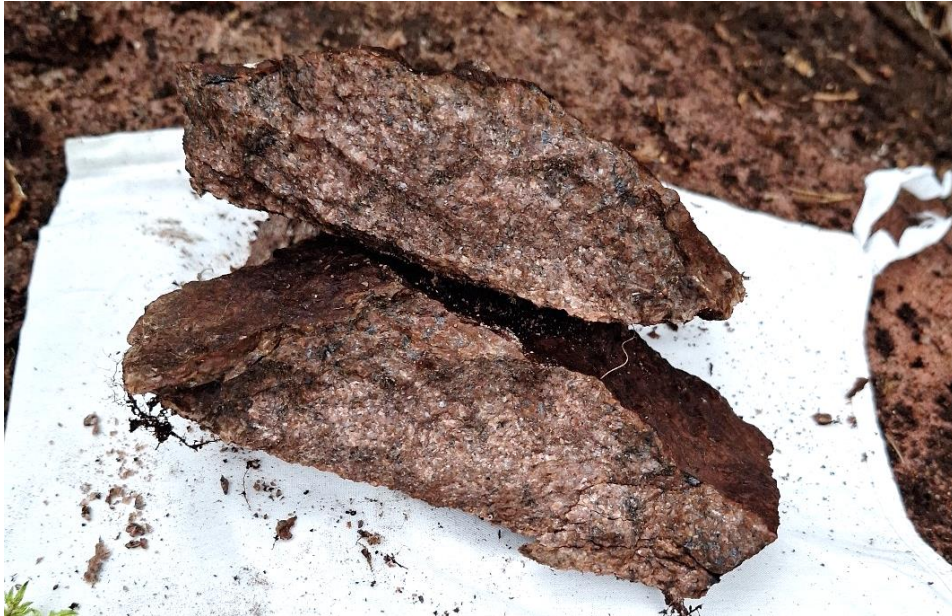
Figure 2: Photograph of magnetite-poor red HREE-bearing syenite intrusive at Melson Sample MEJFG06 that returned 0.6% TREO
