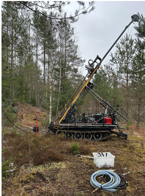
Figure 1: Small footprint diamond drill rig on site ready to commence drilling
