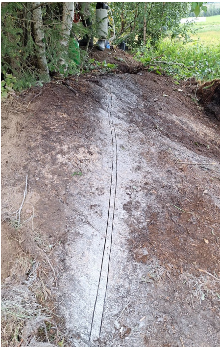
Figure 1: (left) Photograph of diamond cut channel at Orrvik facing south-southeast across strike; and (right) close up of one channel sample interval showing visible spodumene (sp) from channel sample OCSJF06 assaying 2.4% Li 2 O
