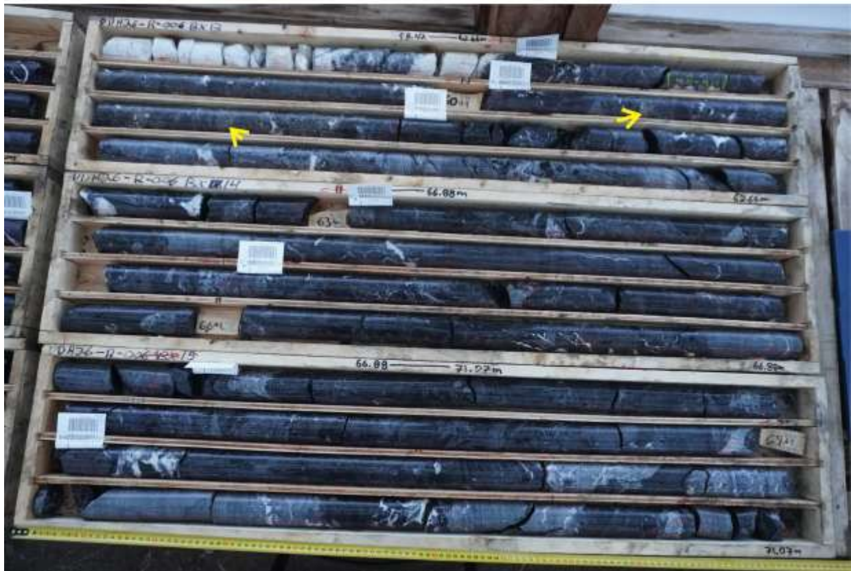
Figure 3 (continued): Core trays (wet) from DDH26-PR-006 (45.65–58.42m, top; 58.42–71.07m, bottom), Pad 2. Yellow arrows indicate clusters of high sphalerite abundance; the yellow box marks the core shown in Figure 4 , left. Mineralised intervals are visual observations only; assays pending.
