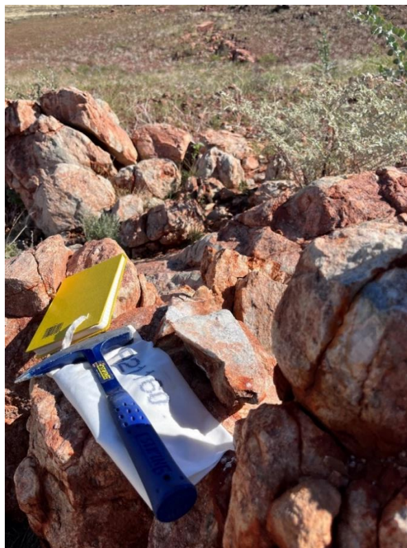
Figure 3: Pegmatite outcrop at rock sample R21160 location, with further pegmatite outcrops along strike (in background)
