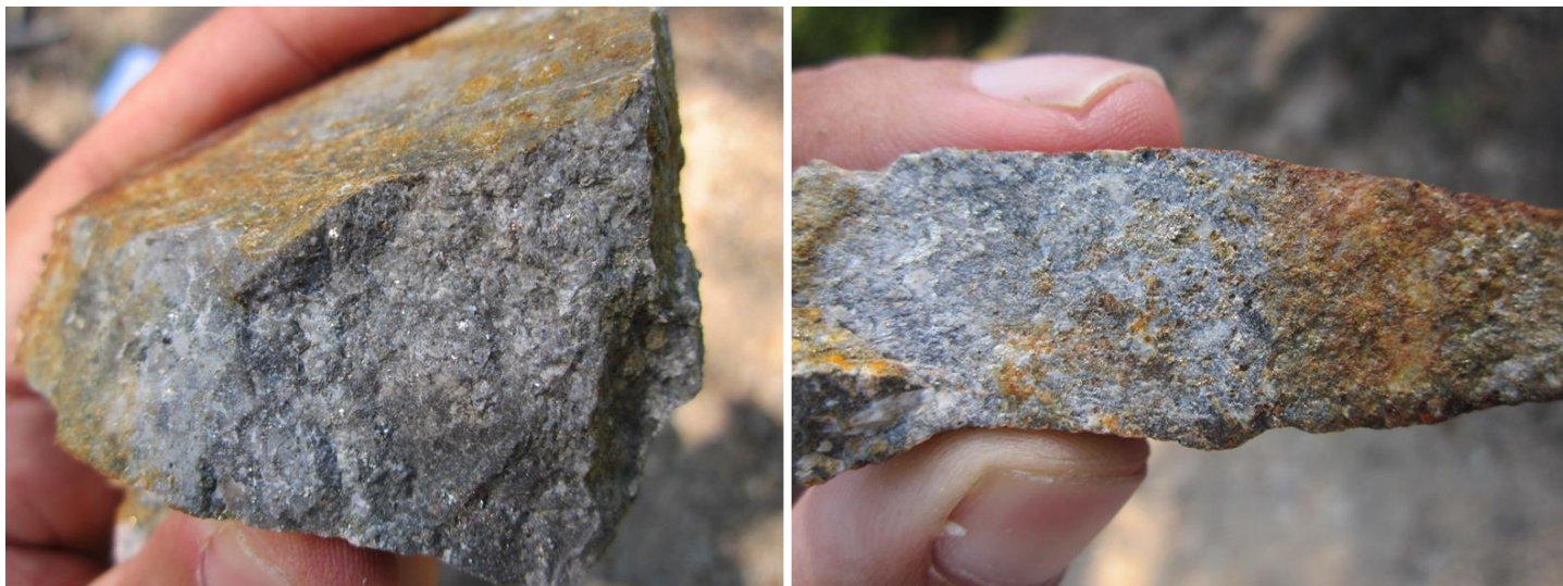
Figure 12 – Disseminated Pyrite, Chalcopyrite and Galena sulphide mineralisation. Mineralisation composes an estimated 0.5 – 1.5% of sample mass
