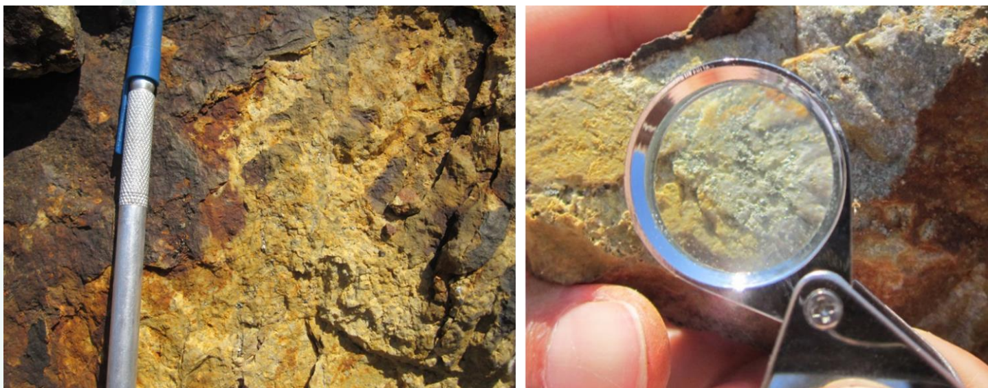
Figure 13 - Pyrite sulphide mineralisation (disseminated and veinlets), within a propylitic altered host rock. The sulphide content is estimated up to 2%
