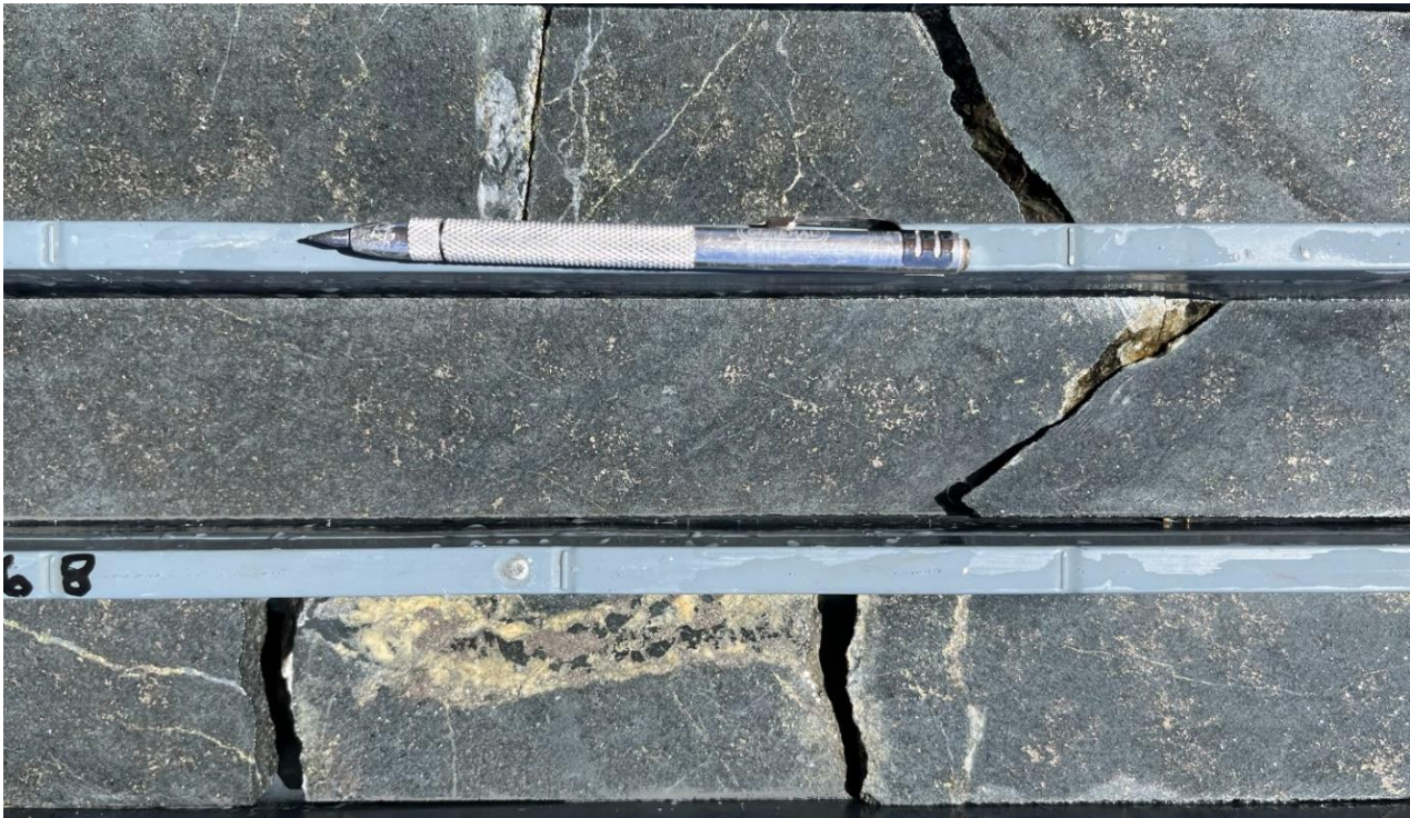
Figure 2: 22B1DD001 (54.28-77.00 metres – cut NQ core 61.1mm diameter) incl. 4.0m @ 2.63% Ni Eq from 73.0m. Strongly mineralised pyroxenite with fine-grained pyrrhotite and chalcopyrite occurring as disseminated mineralisation.
