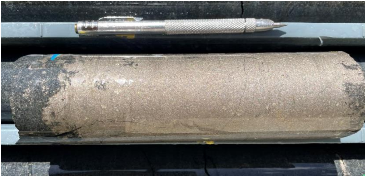
Figure 7: 22B2DD006 (86.7-87.0m interval – NQ core 47.6mm diameter) 0.3m @ 2.98% Ni Eq Strongly mineralised serpentinised ultramafic rock (pyroxenite) with fine-grained massive pyrrhotite with coarse minerals of pentlandite.
