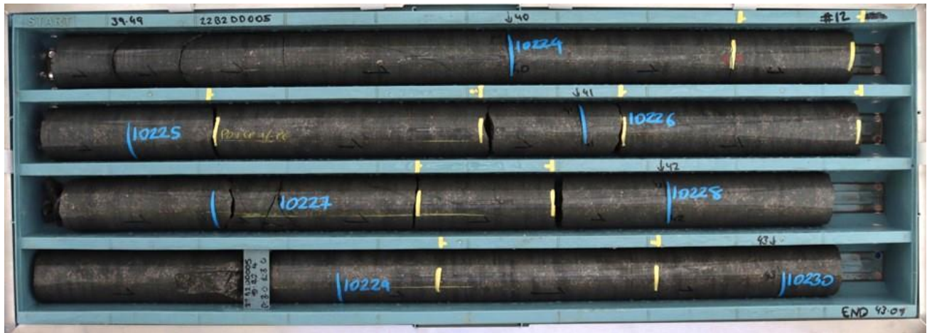
Figure 9: 22B2DD005 (38-45.05m – HQ core 61.1mm diameter) incl. 2.0m @ 3.14% Ni Eq from 41.5m
