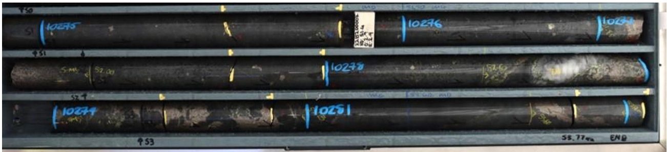
Figure 8: 22B2DD007 (50.00 – 53.77m interval – NQ core 47.6mm diameter) incl. 0.9m @ 5.19% Ni Eq from 52.35m Mineralised dolerite with semi-massive to interstitial sulphide mineralisation, predominantly pyrrhotite with lesser amounts of pentlandite and chalcopyrite.
