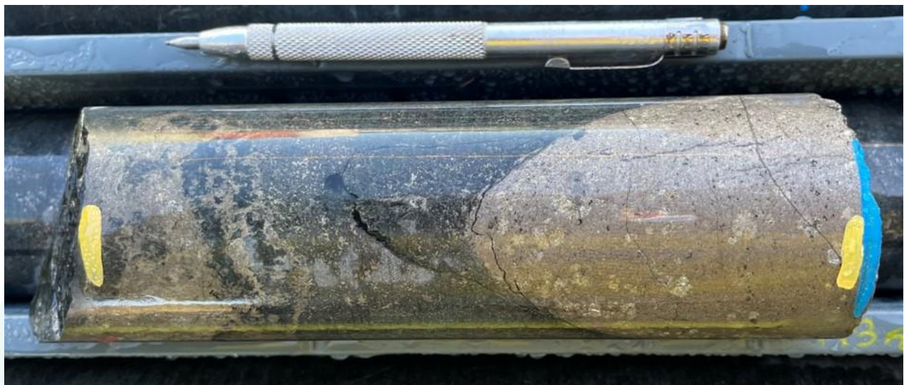
Figure 10: 22B2DD008 (112.0-112.5m interval – NQ core 47.6mm diameter) 0.5m @ 2.75% Ni Eq
