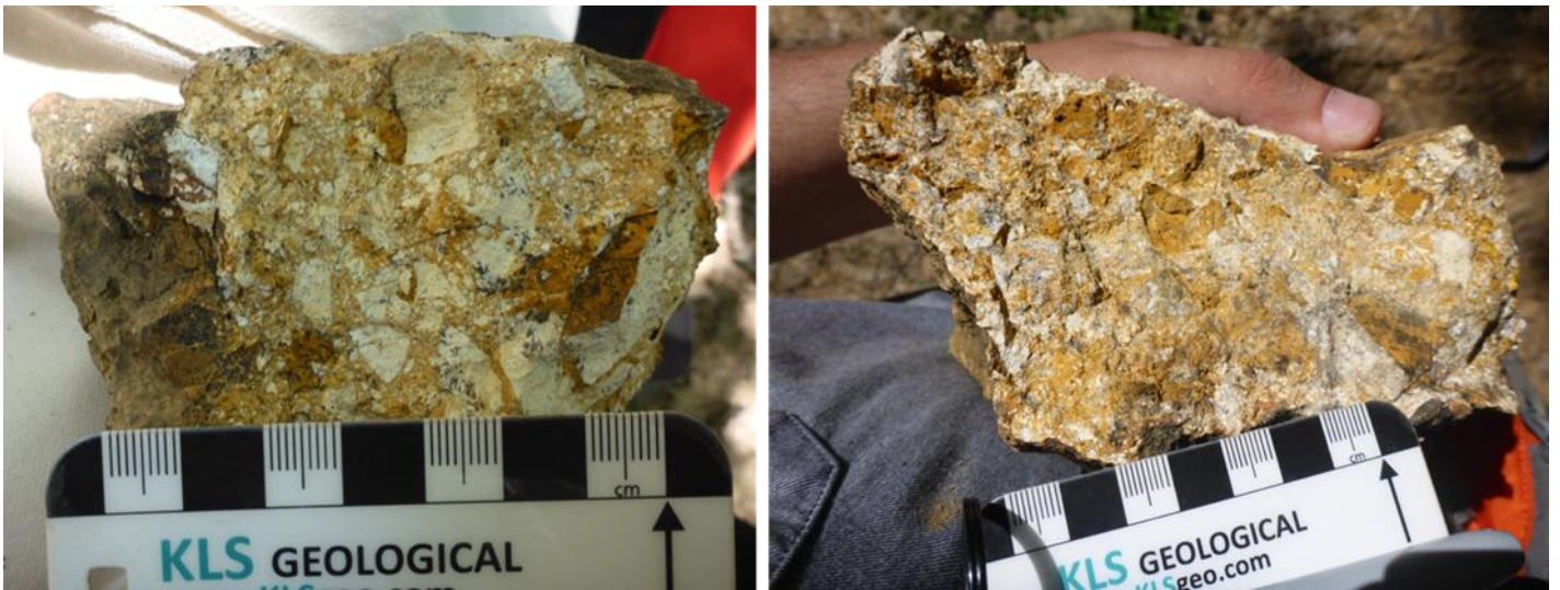
Figure 4 - Hydrothermal / tectonic breccia on the contacts of rhyolitic dykes at Belopoltsi target
