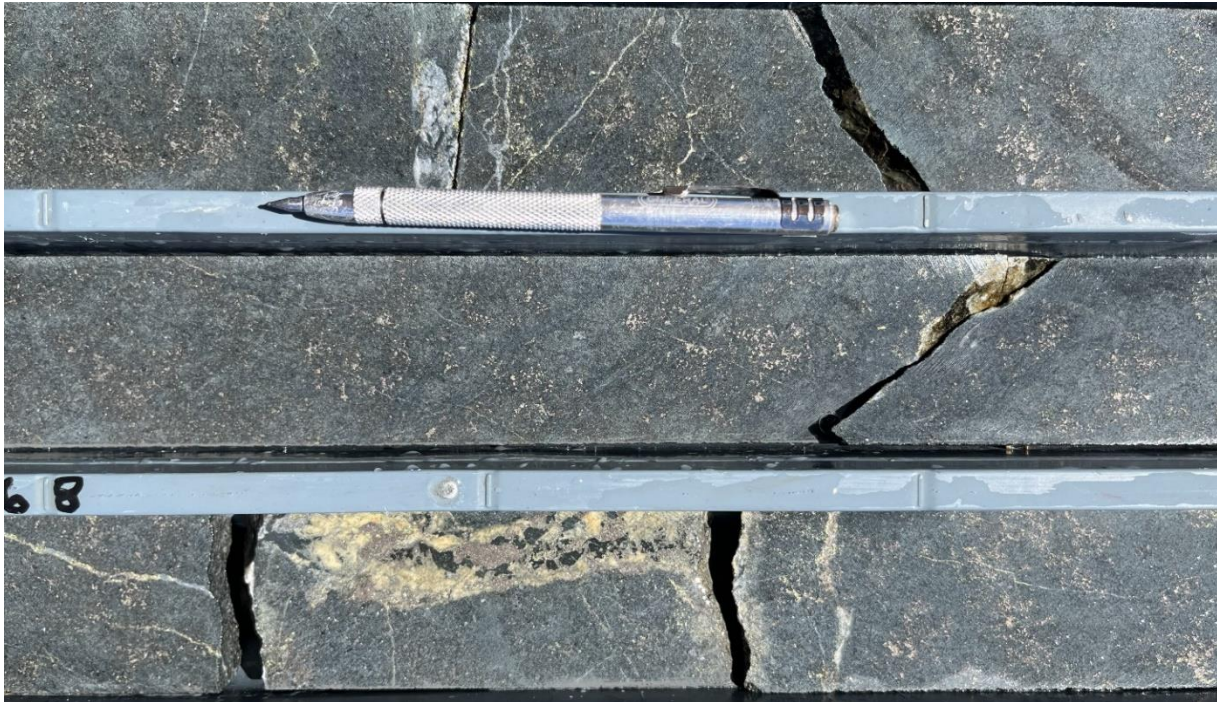
Figure 3: 22B1DD001 (54.28-77.00 metres – cut NQ core 61.1mm diameter) Strongly mineralised pyroxenite with fine-grained pyrrhotite and chalcopyrite occurring as disseminated mineralisation, within a 22.72 metre zone of sulphide mineralisation. 1
