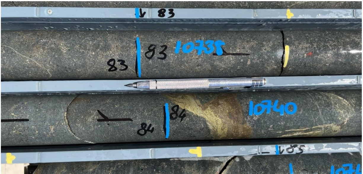
Figure 1: 22B1DD002 (included in the 76.8-85.4 metre interval – NQ core 47.6mm diameter). Strongly mineralised pyroxenite with fine-grained pyrrhotite and chalcopyrite with lesser pyrite, including a band of massive chalcopyrite and oxidised pyrrhotite between 84.0-.84.1m, Within a 20.7 metre zone of sulphide mineralisation. 1 Mineralisation is mottled and massive.
