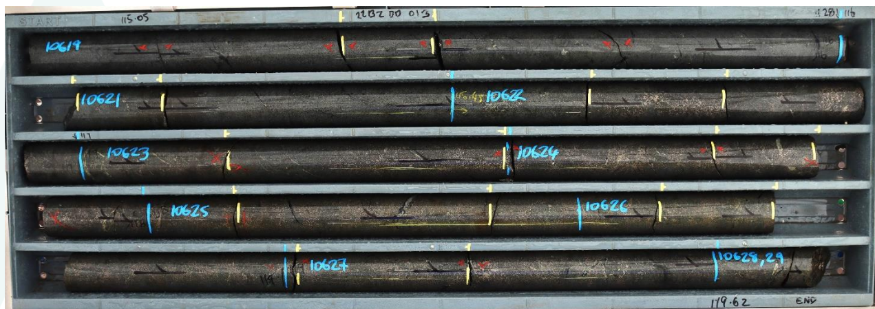
Figure 1: 22B2DD013 (115.05-119.62m – NQ core 47.6mm diameter) incl. 3.1m @ 3.83% Ni Eq from 116.4m Strongly mineralised dolerite with densely disseminated fine-grained pyrrhotite, chalcopyrite, and pentlandite.
