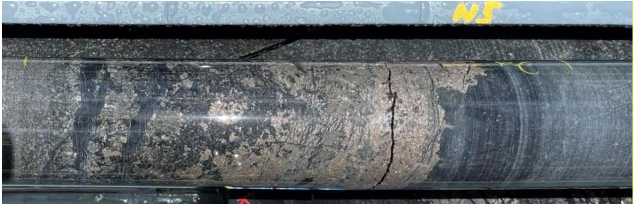
Figure 3: 22B2DD009 (34.9-35.1m – NQ core 47.6mm diameter) Strongly mineralised pyroxenite with fine-grained semi-massive pyrrhotite, pyrite, and pentlandite within a 39.3m zone of sulphide mineralisation. 1
