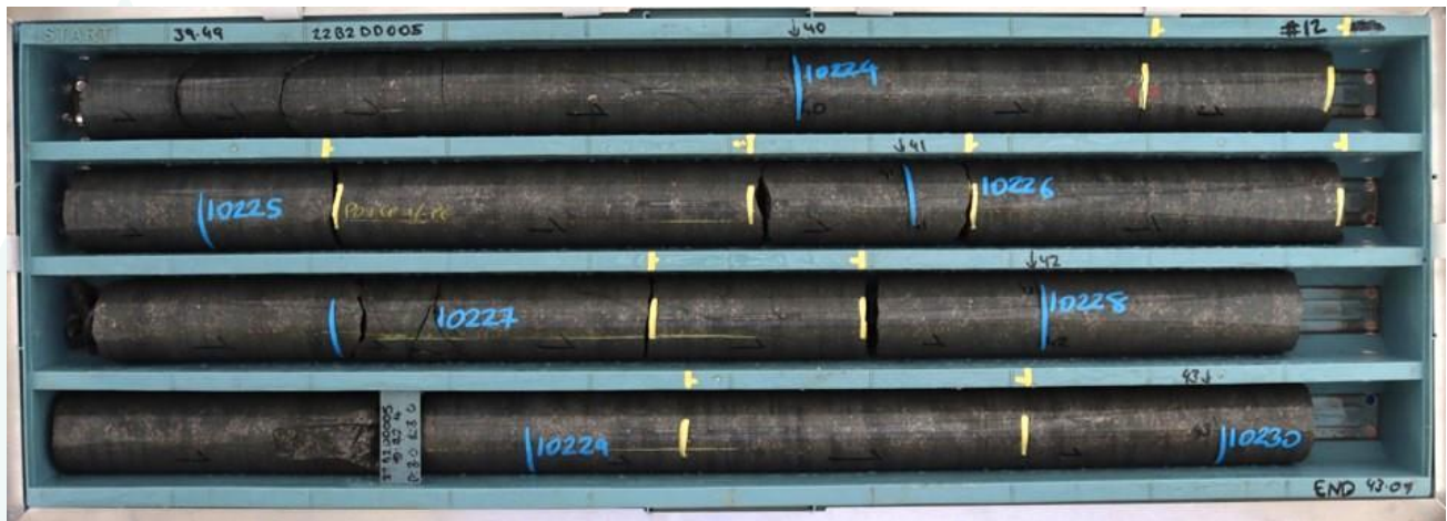
Figure 4: 22B2DD005 (38-45.05m – HQ core 61.1mm diameter) Strongly mineralised dolerite with coarse disseminated angular blebs of fine-grained pyrrhotite, chalcopyrite, and pentlandite within a 27.8m zone of sulphide mineralisation. 1
