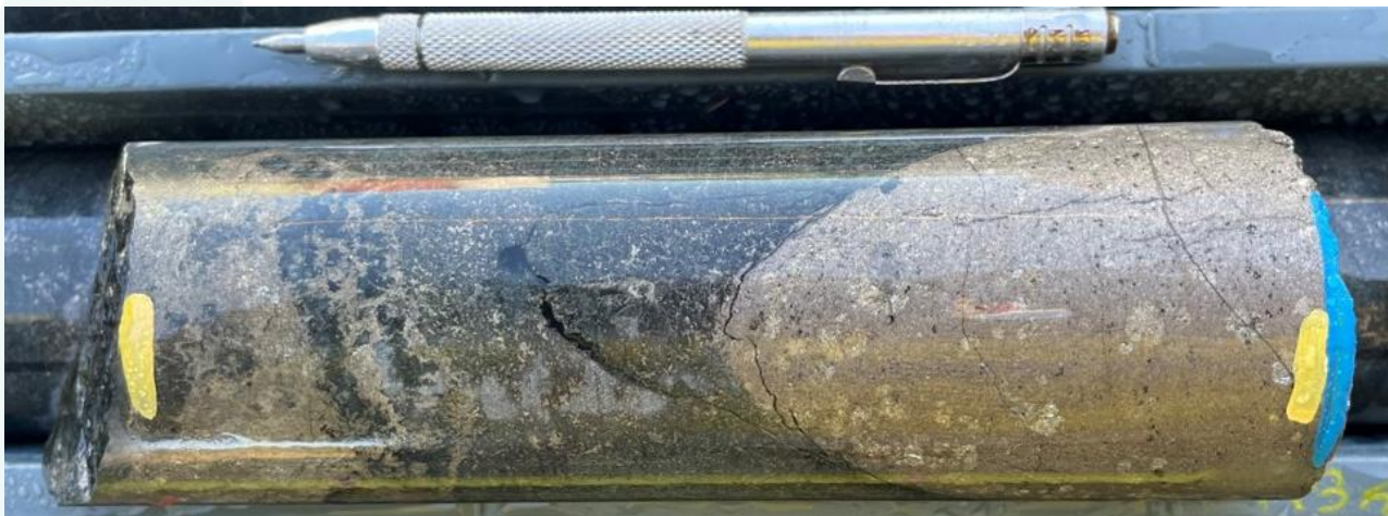
Figure 1: 22B2DD006 (86.7-86.9m interval – NQ core 47.6mm diameter). Strongly mineralised ultramafic rock (pyroxenite) with fine-grained massive pyrrhotite with coarse minerals of pentlandite. Within a 35.1m zone of sulphide mineralisation. 1
