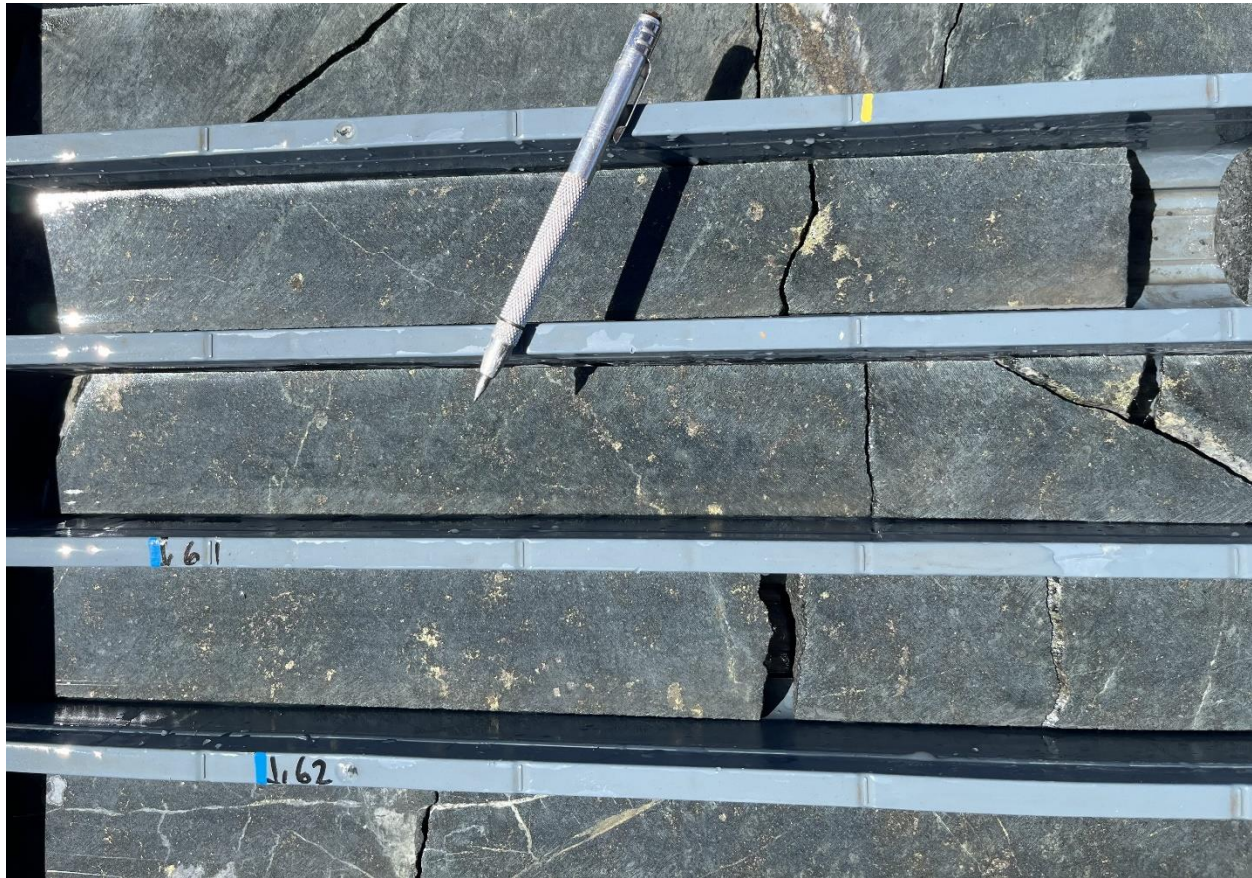
Figure 4: 22B1DD013 (58.7 – 63m interval – NQ core 47.6mm diameter). Mineralised dolerite with fine-to-coarse grained blebby disseminated pyrrhotite and chalcopyrite, with lesser pentlandite. Within a 20.3 metre zone of sulphide mineralisation. 1
