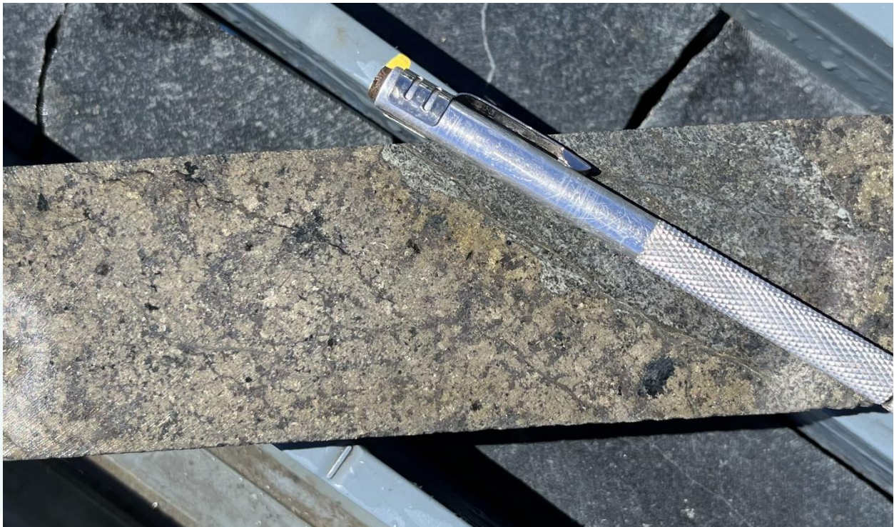
Figure 3: 22B1DD011 (17.84 – 18.2 metre interval – NQ core 47.6mm diameter). Strongly mineralised pyroxenite with fine-grained massive pyrrhotite and pentlandite, with lesser chalcopyrite mineralisation, within a 22.36 metre zone of sulphide mineralisation. 1
