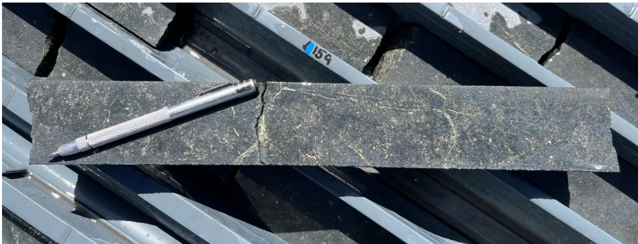
Figure 1: 22A1DD003 (156 - 165 metre interval – NQ core 47.6mm diameter). Strongly mineralised dolerite with fine-grained disseminated pyrrhotite-chalcopyrite mineralisation, within a 20.8 metre zone of sulphide mineralisation. 1
