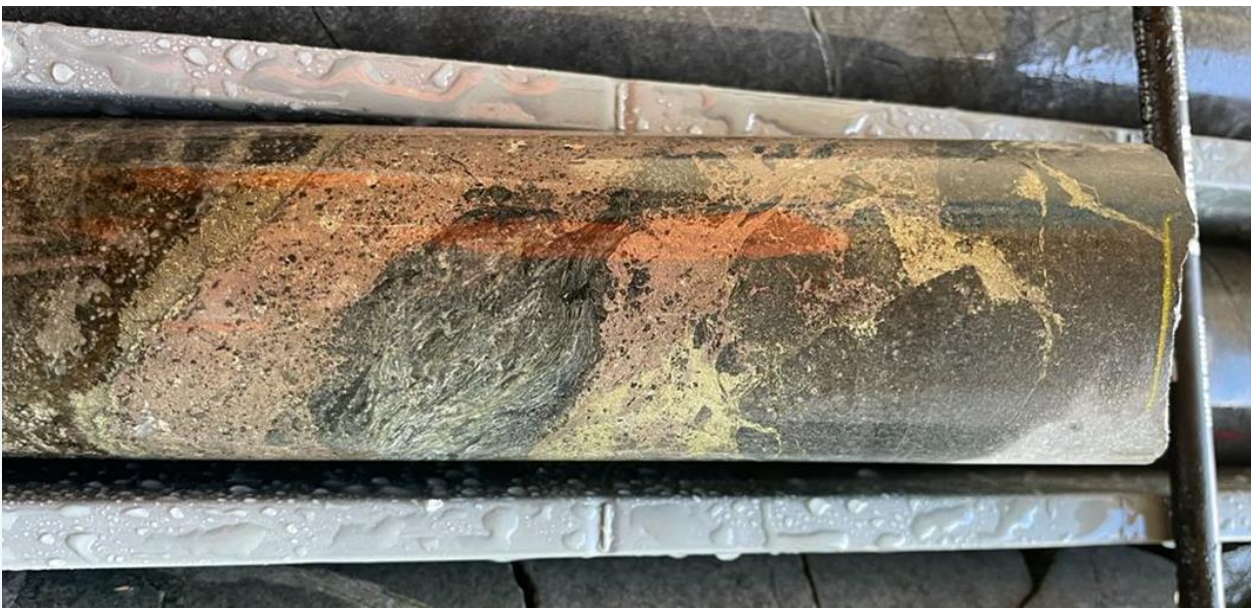
Figure 1: 22B2DD003 (26.8 -27.0 metre interval – NQ core 47.6mm diameter). Strongly mineralised dolerite with fine-grained pyrrhotite, chalcopyrite and coarse minerals of pentlandite. Mineralisation is semi-massive and interstitial. Within a 29.35 metre zone of sulphide mineralisation. 5
