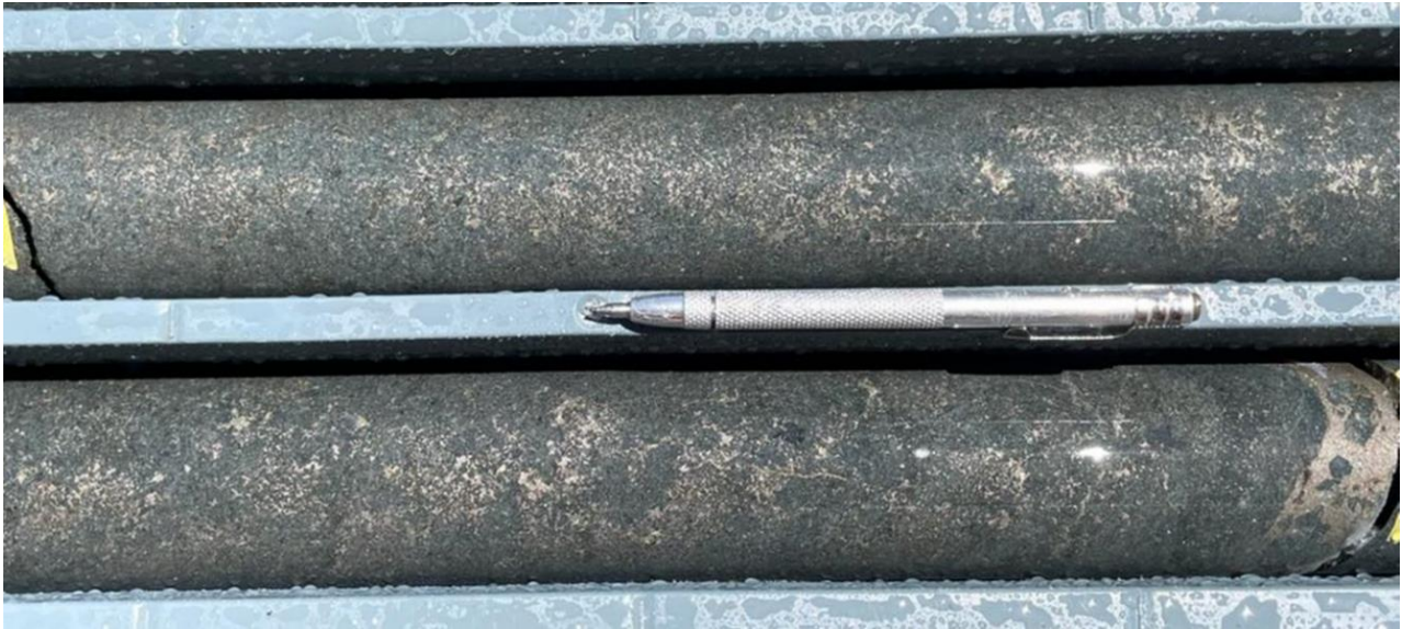
Figure 4: 22B2DD003 (40-42 metres – NQ core 47.6mm diameter) Strongly mineralised dolerite with disseminated angular blebs of fine-grained pyrrhotite and pentlandite with minor chalcopyrite, within a 29.35 metre zone of sulphide mineralisation. 5
