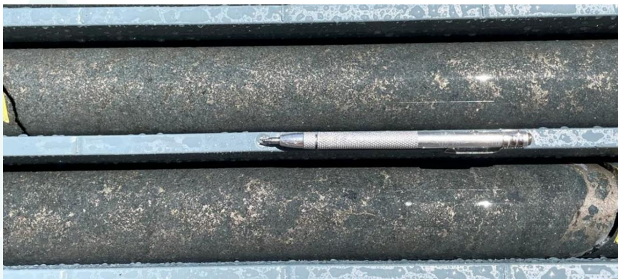
Figure 6: 22B2DD003 (40.2-42.0 metres – NQ core 47.6mm diameter) 1.8m @ 2.32% Ni Eq Strongly mineralised dolerite with disseminated angular blebs of fine-grained pyrrhotite and pentlandite with minor chalcopyrite.
