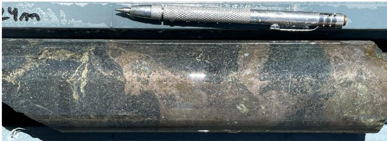
Figure 3: 22B2DD001 (61.0 - 61.4 metre interval – NQ core 47.6mm diameter) 0.4m @ 2.48% Ni Eq Strongly mineralised dolerite with fine-grained massive to semi-massive pyrrhotite mineralisation with coarse minerals of pentlandite and chalcopyrite.
