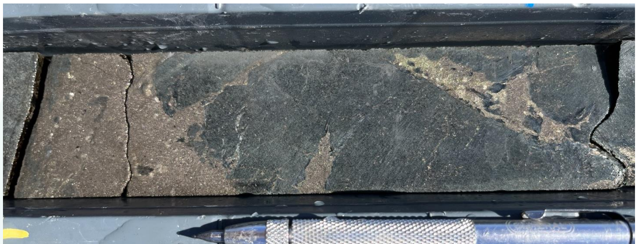
Figure 5: 22B2DD012 (116.5-116.8 interval – NQ core 47.6mm diameter). Strongly mineralised dolerite with fine-grained massive to patchy pyrrhotite with pentlandite. Within a 23.5m zone of sulphide mineralisation. 1
