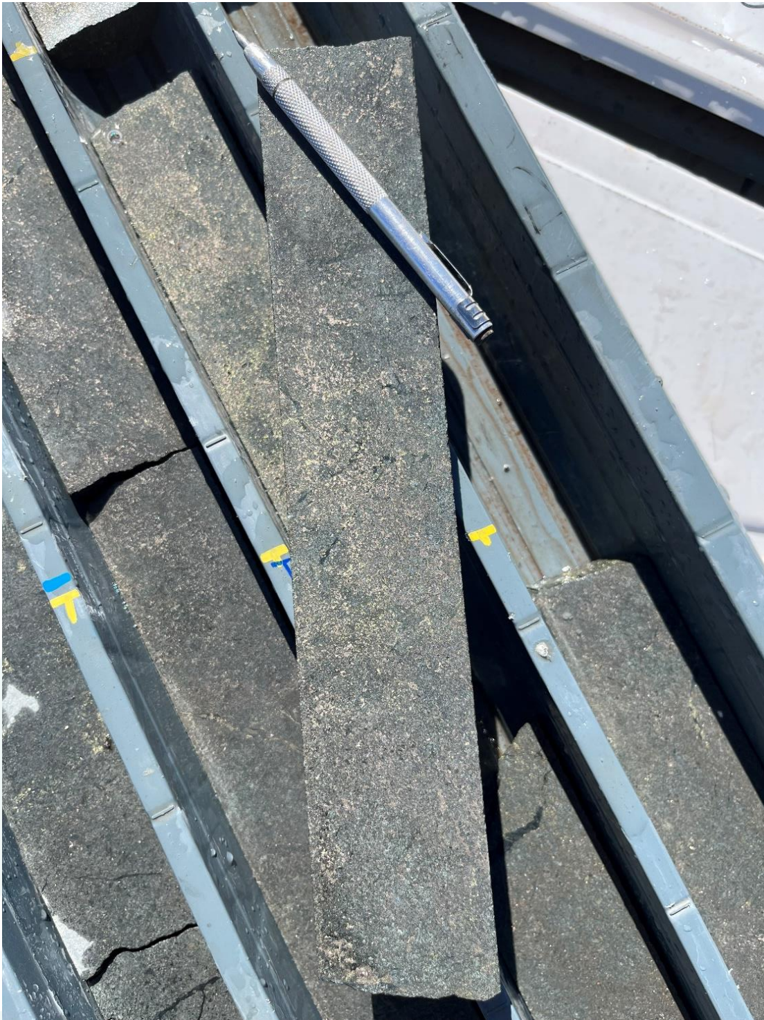
Figure 7: 22B2DD013 (116.45-120.2 – cut NQ core 47.6mm diameter) Strongly mineralised dolerite with coarse-grained disseminated pyrrhotite, chalcopyrite, and minor pentlandite within an 18.54m zone of sulphide mineralisation. 1
