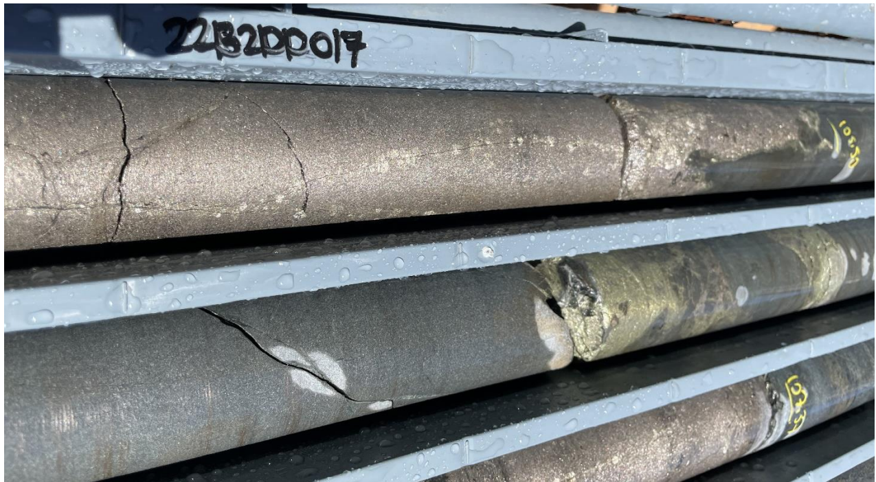
Figure 4: 22B2DD017 (105.08-107.37 interval – NQ core 47.6mm diameter). Detailed image of Figure 2 above showing the coarse pentlandite grains, along a fracture, within the fine-grained massive pyrrhotite. Within a 38.94m zone of sulphide mineralisation. 1
