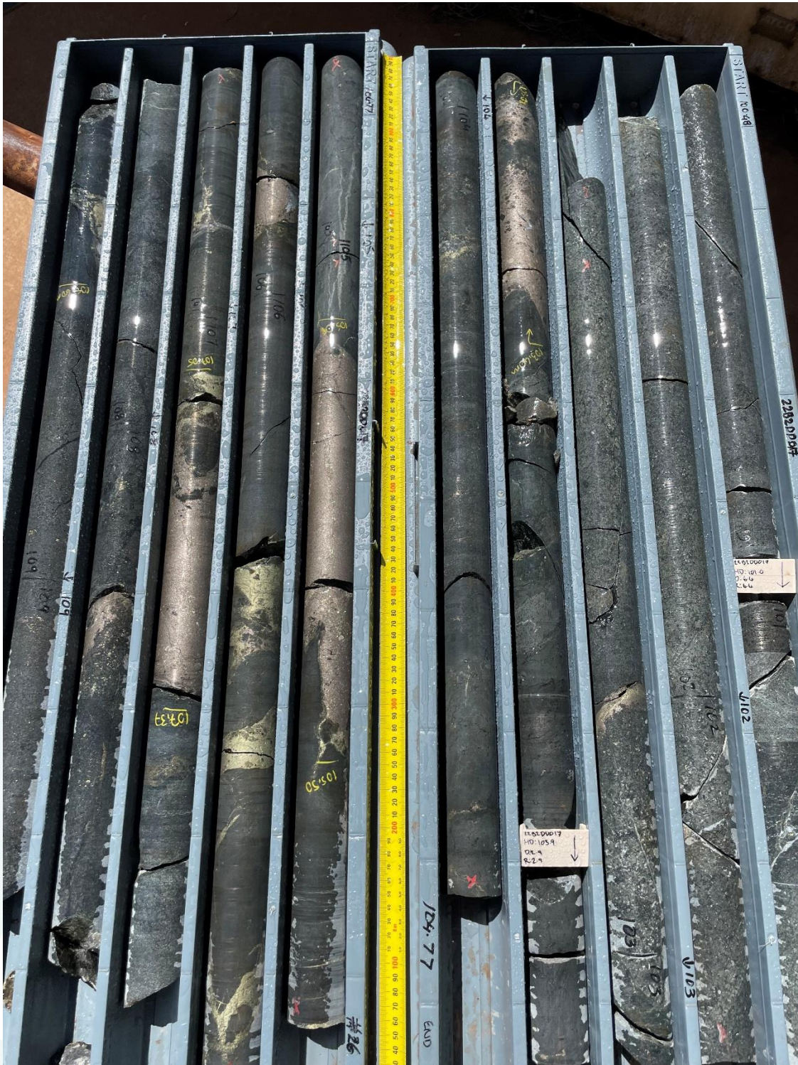
Figure 1: 22B2DD017 (100.16-109.5m interval – NQ core 47.6mm diameter). Strongly mineralised dolerite with bands of fine-grained massive pyrrhotite and coarser pentlandite, along with a zone of chalcopyrite-pyrrhotite-pentlandite, within fine-grained disseminated pyrrhotite mineralisation. Within a 38.94m zone of sulphide mineralisation. 1
