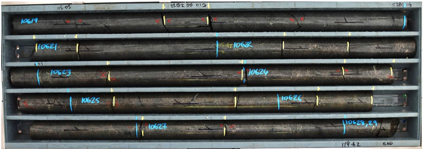
Figure 1: 22B2DD013 (115.05-119.62m – NQ core 47.6mm diameter) incl. 3.1m @ 3.83% Ni Eq from 116.4m Strongly mineralised dolerite with densely disseminated fine-grained pyrrhotite, chalcopyrite, and pentlandite 4 .
