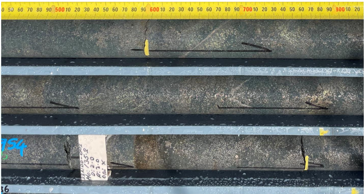
Figure 4: 22A1DD002 (133.5-135.5m interval – NQ core 47.6mm diameter). Mineralised pyroxenite with fine-to-coarse grained disseminated pyrrhotite and chalcopyrite. Within a 15.9 metre zone of sulphide mineralisation. 1
