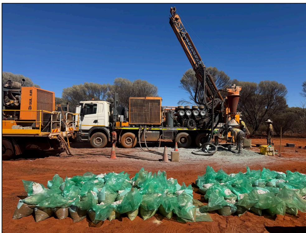
Figure 1: RC drilling rig in operation at the Goodenough Gold Deposit, East Menzies Gold Project, WA
