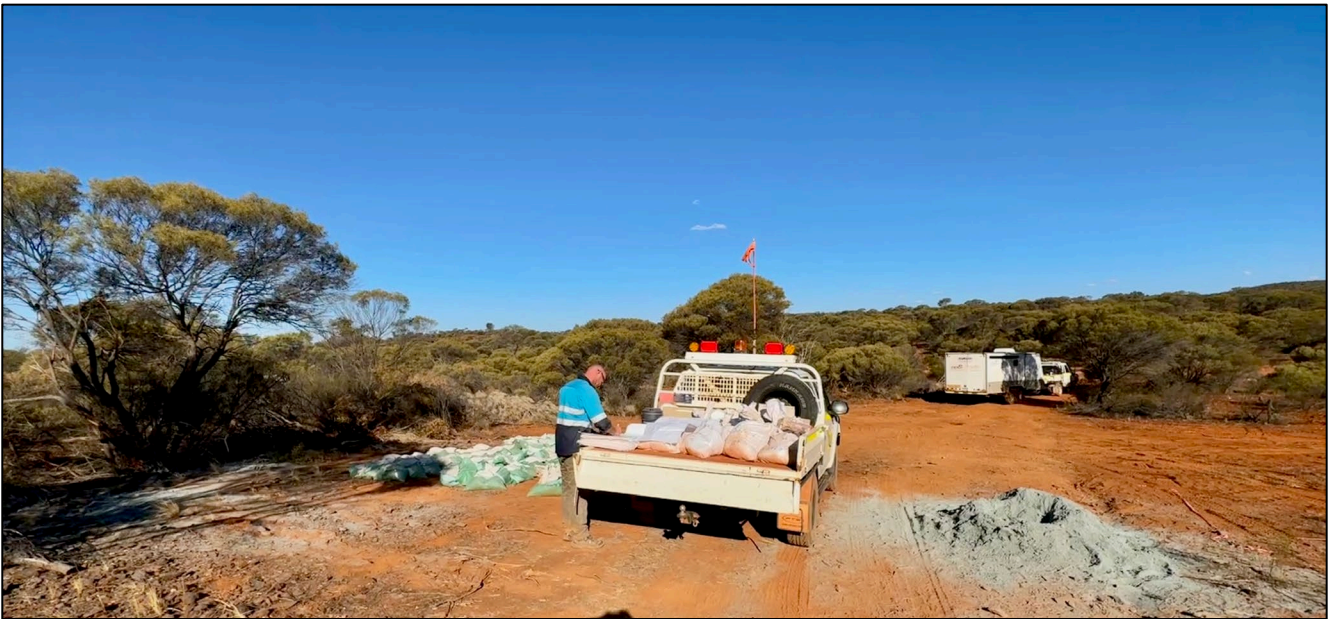
Figure 2: RC samples from drilling at the Goodenough Gold Deposit ready for dispatch
