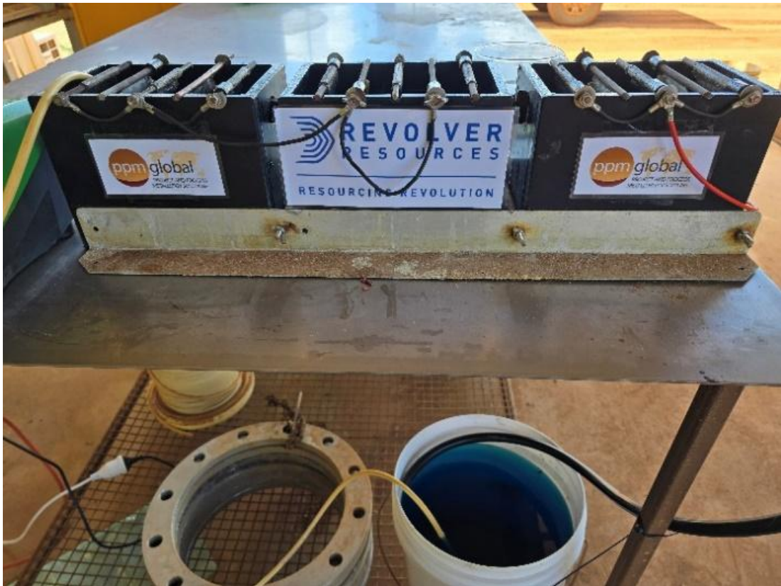
Figure 11: Scale EW cell used for plating copper cathode from Dianne Ore
