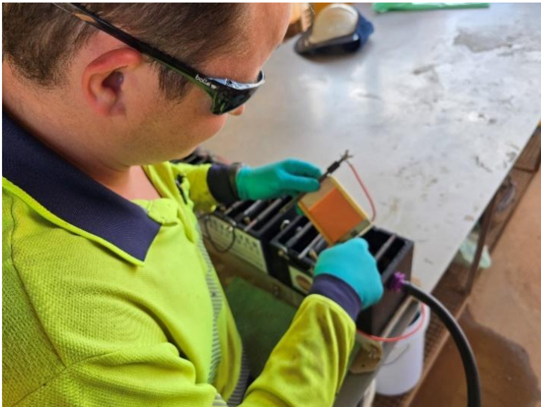
Figure 12: Cathode produced from Dianne Ore
