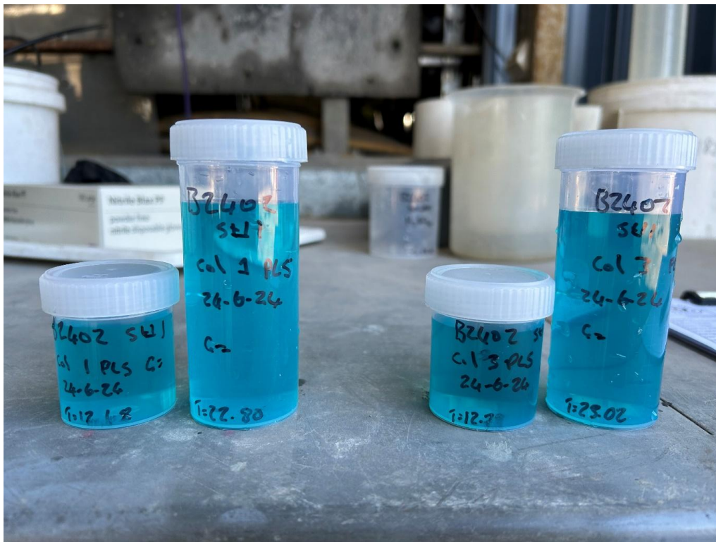
Figure 5: Pregnant leach solution obtained from column leach testwork
