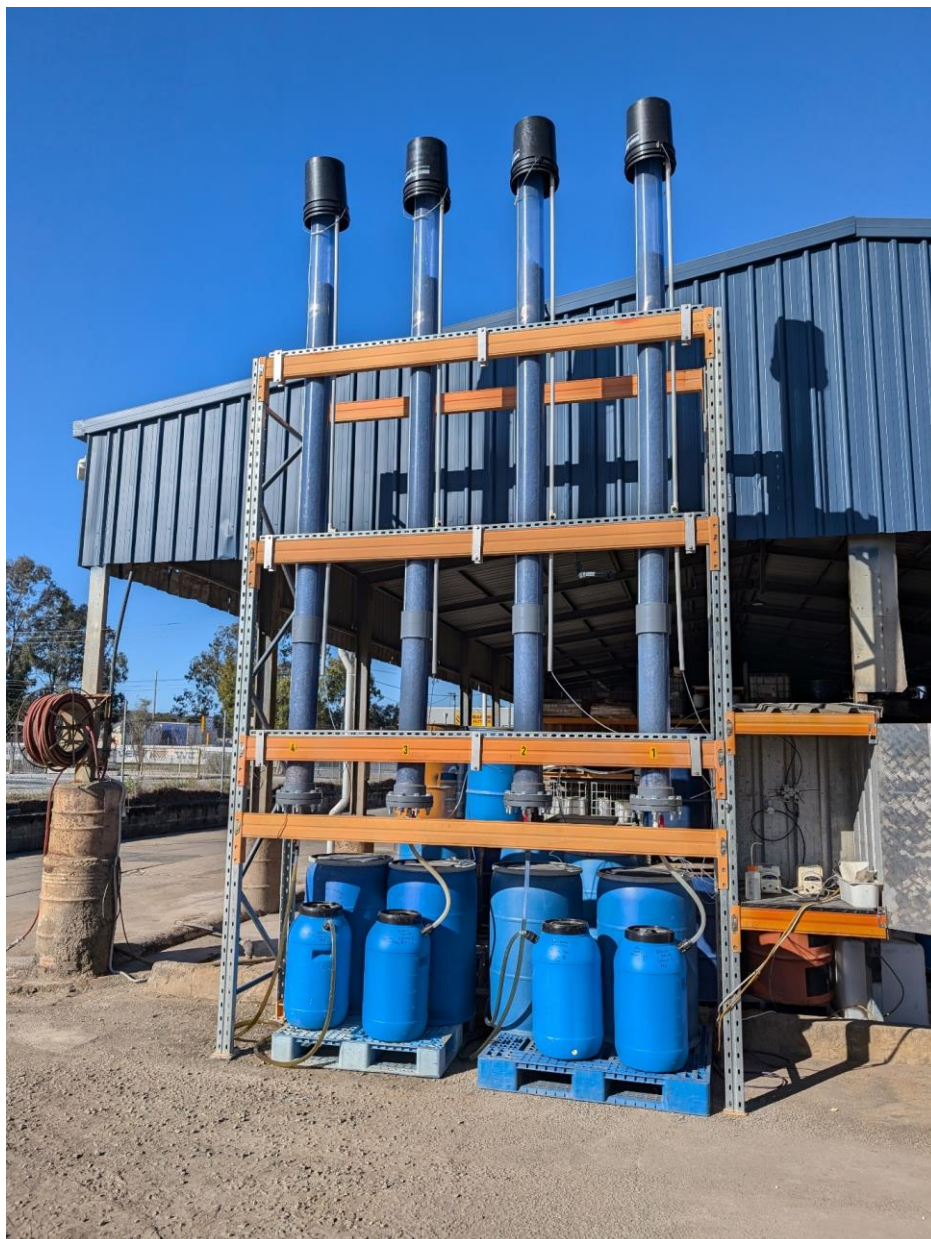
Figure 2: Four column leach test configuration
