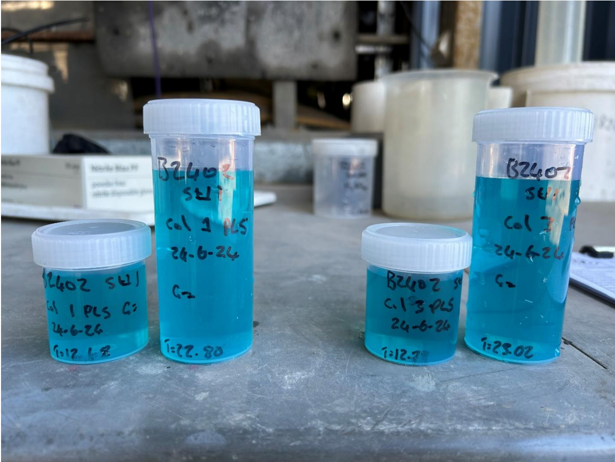
Figure 4: Pregnant leach solution obtained from column leach testwork
