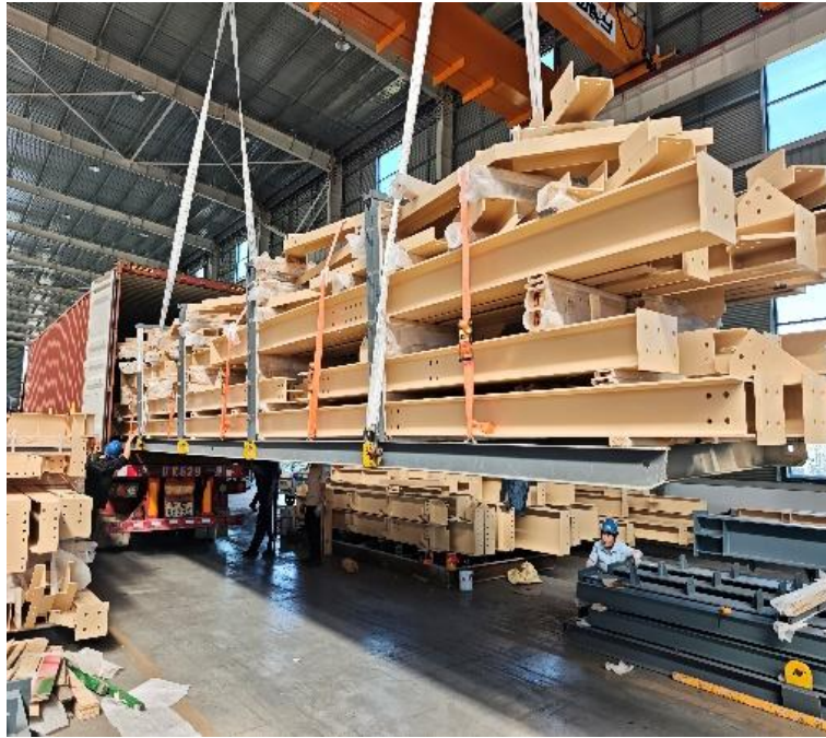
Figure 11 – Structural steel loading for shipment
