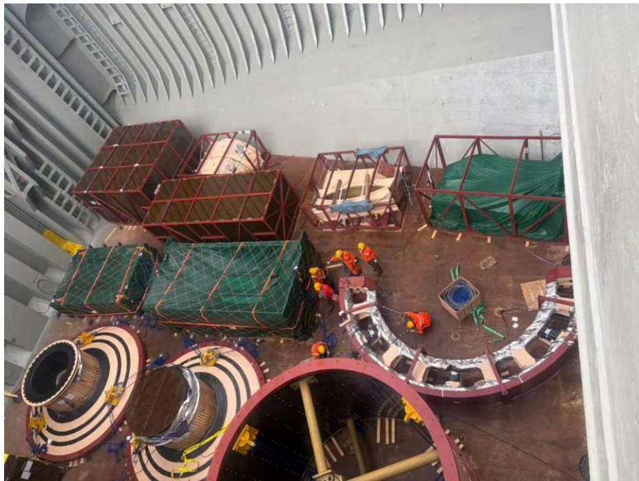
Figure 10 – Ball mill and components loaded in ship for transport
