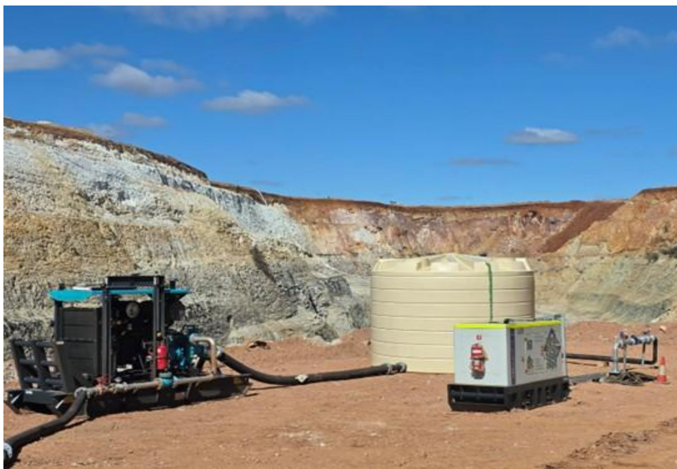
Figure 2 – Youanmi Main initial UG dewatering setup
