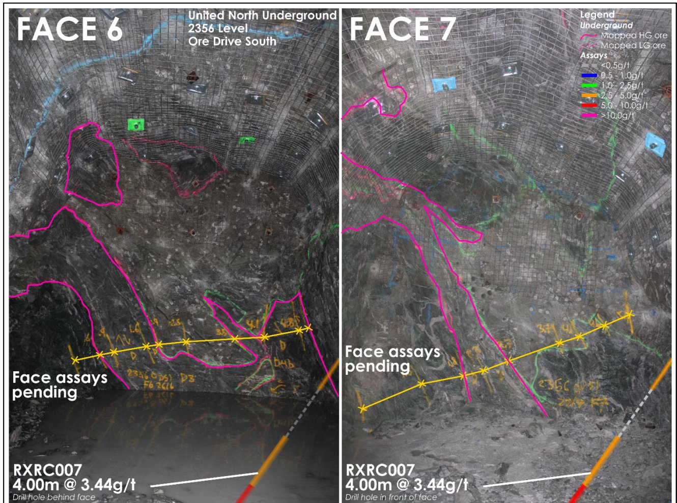
Figure 8 – United North 2356mRL ore drive south face 6 & 7, mapped shear zone vs. nearest drill hole comparison
