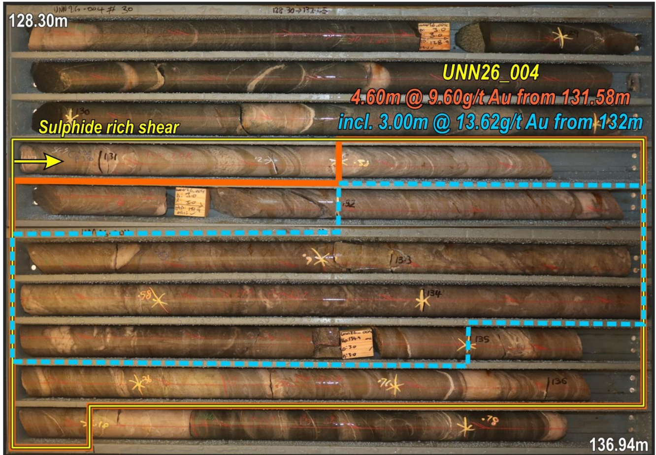
Figure 3 – United North underground diamond drill hole UNN26_004 logged shear and significant intercept
