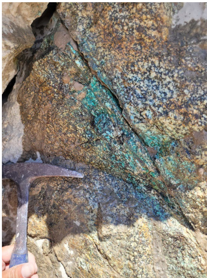
Figure 4: Cu oxides adjacent to quartz veining and fractures in porphyritic quartz granodiorite with coarse biotite crystals.
