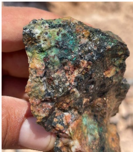
Figure 3; Tourmaline breccias 1 at Chancho al Palo with copper oxides in tuffs – eastern porphyry zone (Coordinates 254930E, 8068540N).
