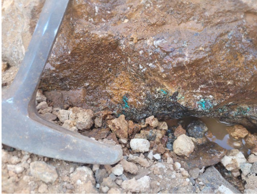
Figure 4; Copper oxides 1 in structures associated with calcic, sodic, and epidote alteration with specularite veining – western IOCG zone, Chanco al Palo (Coordinates 254478E, 8068009N).
