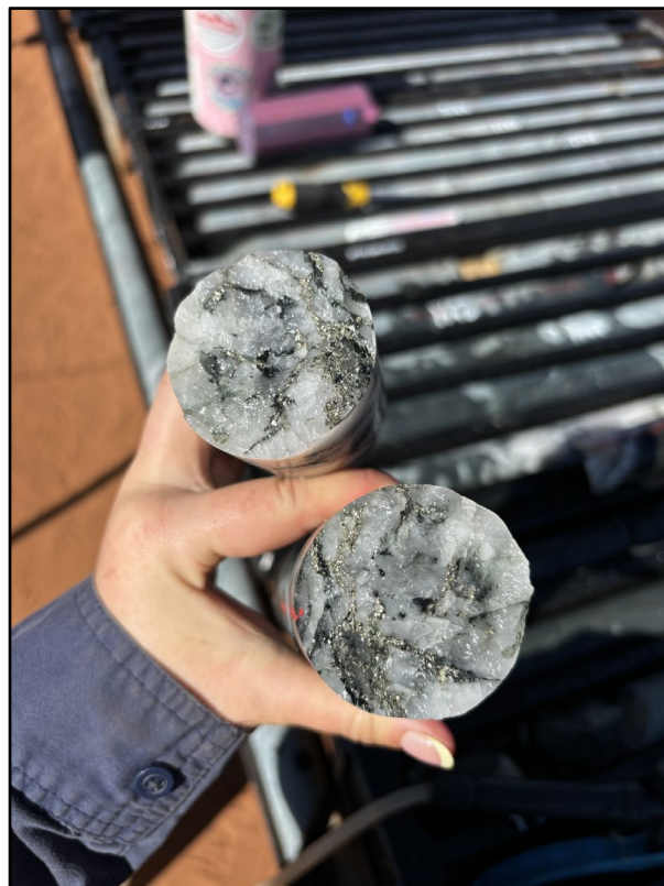
Figure 5: SMXDD003 – quartz, pyrite, pyrrhotite at 775m. No significant results returned
