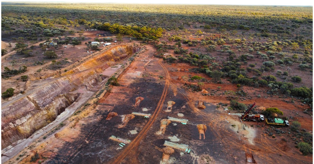
Picture 1: RC drill rig on site at Zelica targeting depth extensions of known mineralisation below pre-existing shallow open pit on the left (looking NNW)
