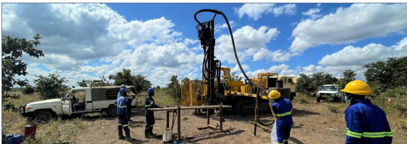
Figure 5: Air-core (AC) drilling at Kasiya in May 2022.
