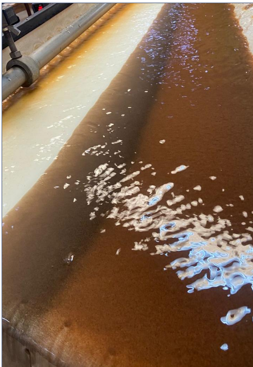
Figure 3: Monazite rich HMC clearly observable from gravity separation of non-conductor tailings (taken from samples disclosed in this announcement)
