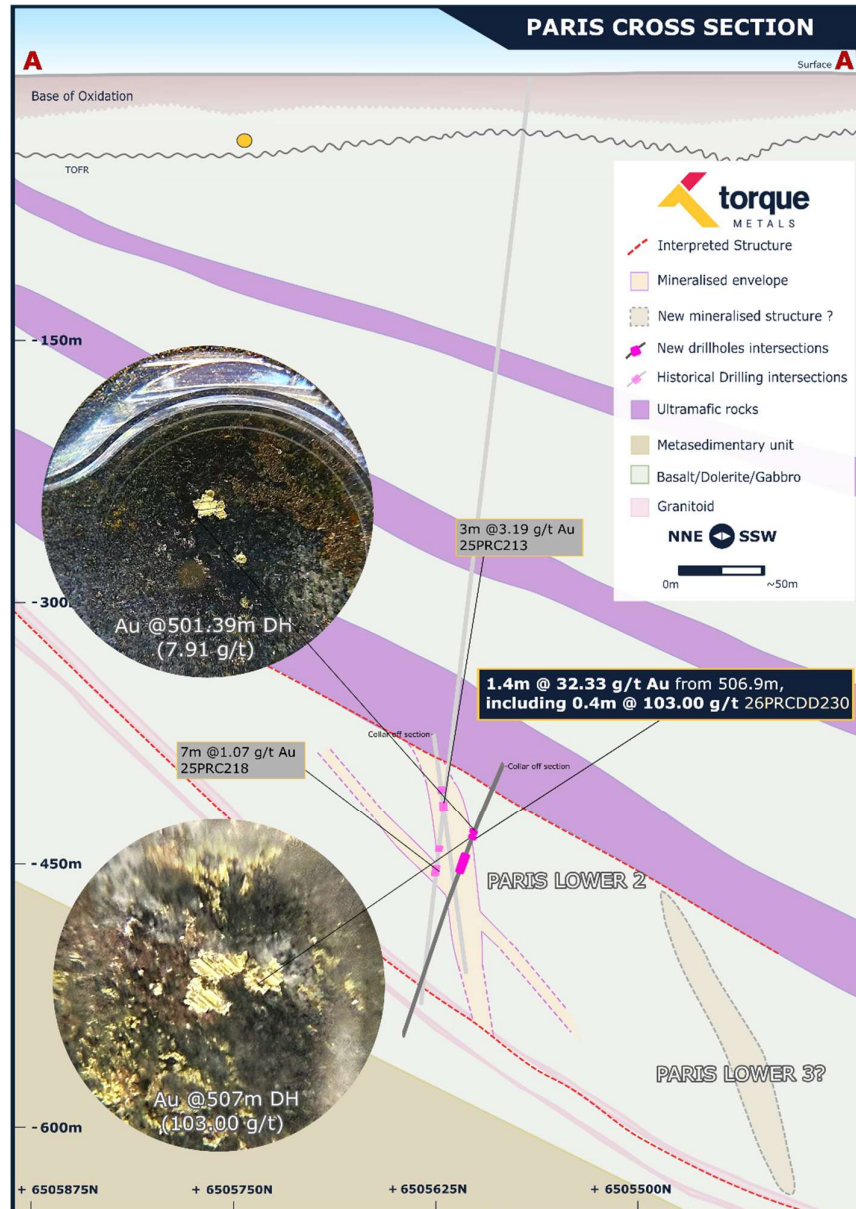
Figure 2: Paris Gold Deposit cross section, highlighting the multi lode system and recent intersections. Visible gold shown above is from hole PRCDD230 and has been assayed, the results of which are reported in this release
