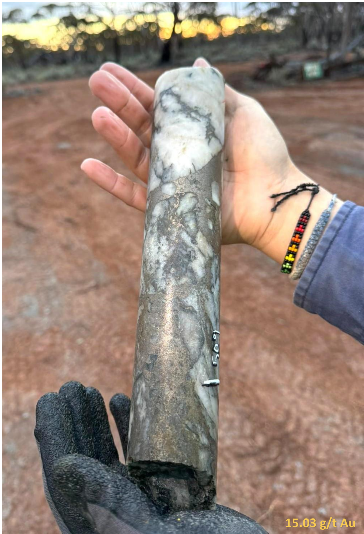
Figure 2 Core at 508.82m to 509.2m (grading 15.03 g/t gold) displaying semi-massive sulphides as pyrrhotite chalcopyrite arsenopyrite breccia with quartz carbonate veining and chlorite alteration. Type of veining and alteration often associated with orogenic gold systems, near structural feeders.
