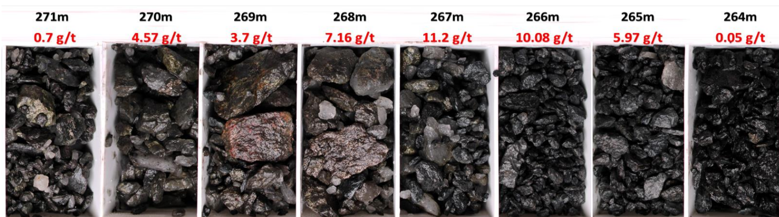
Figure 2 RC drill chips, hole 25PRC174, abundant pyrrhotite, chlorite alteration and quartz carbonate veins including 6m @ 7.1 g/t gold from 265m.
