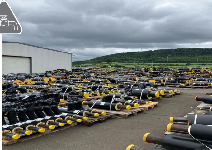
ICPP pipe connections at pipe fabrication yard in Germany.
