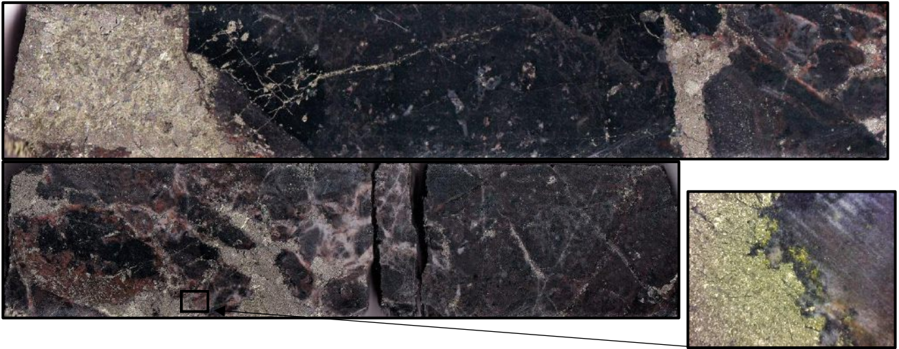
Figure 6: SPD075 556.9 m 206 g/t Au (simple assay sample). Pyrite vein reactivated as a chalcopyrite breccia and a quartz-pyrite-chalcopyrite-carbonate-gold cemented hydrothermal breccia with gold grains adjacent to pyrite (sample is continuous).
