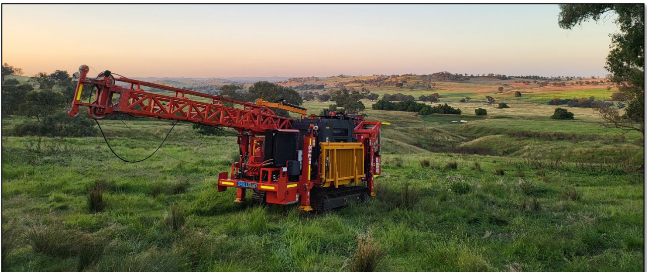
Figure 1: Diamond drill rig collaring hole SPD001 at the Spur Prospect
