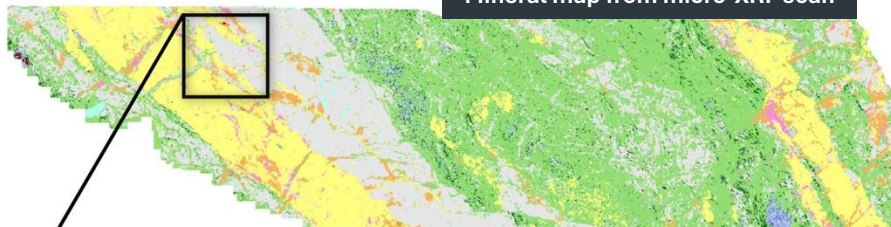
Mineral map from high resolution micro-XRF scan
