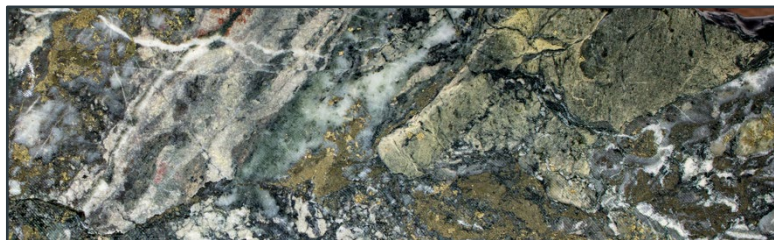
SPRCD037 @ 448-449m 7.06g/t Au. Quartz carbonate sulphide breccias
