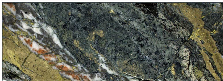
SPRCD037 @ 436-437m 11.6g/t Au. Massive sulphide veins
