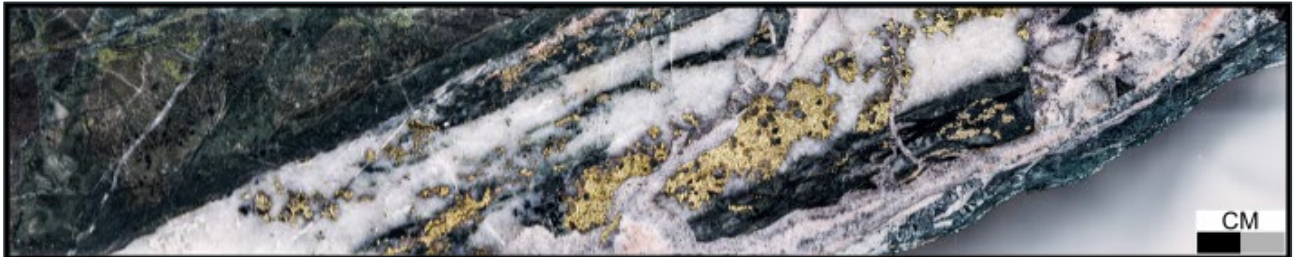
SPD016 144.2 m (Spur, HQ Core). laminated quartz-carbonate-pyrite-chalcopyrite vein hosted in andesite, 13.41 g/t Au.
