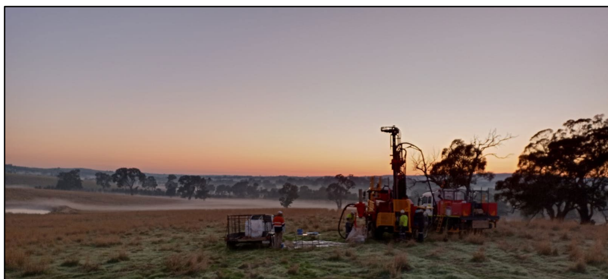
Figure 2: Aircore drill rig collaring hole at the Frankfurt Prospect
