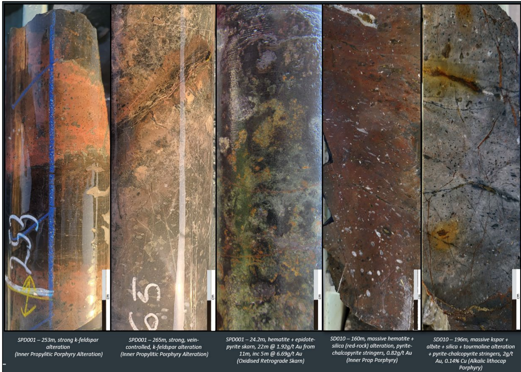
Figure 6: Spur Project. Core photography of representative porphyry alteration types
