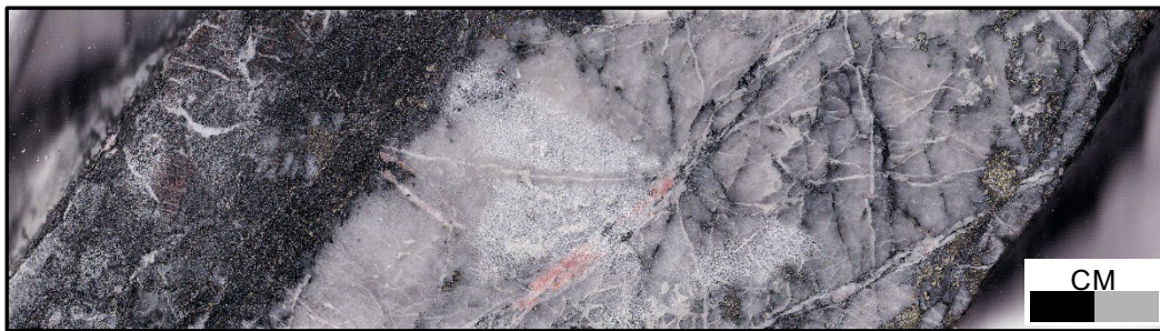
Figure 8 – SPD028 283.7m grading 7.57 g/t Au . Quartz-pyrite-chalcopyrite-magnetite fault zone
