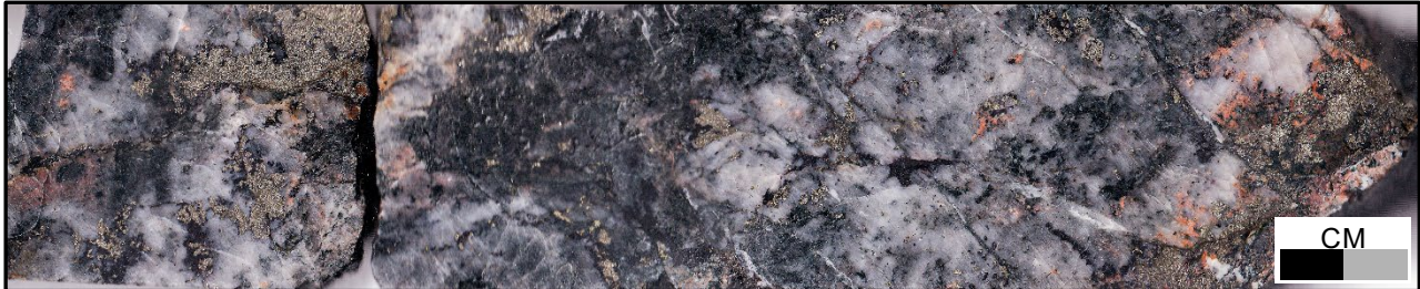
Figure 2 - SPD025 276.1m grading 6.45 g/t Au. Quartz-pyrite-magnetite-chalcopyrite fault zone
