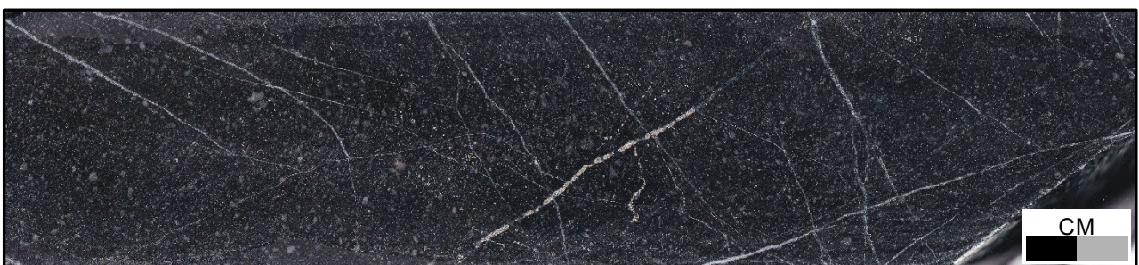
Figure 6 – SPD019W1 481.3m grading 9.66 g/t Au. Andesite with quartz-pyrite veinlets
