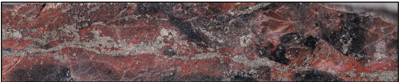
Figure 3 - SPD025 293m grading 13.74 g/t Au. Sulphide veinlets
